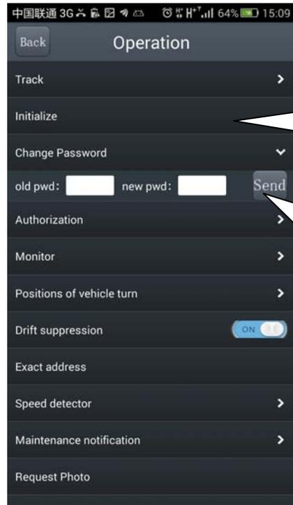
Remarks: "SMS login" version on Android phone can track the positions and show alarm on the map; but "SMS login" version on IOS can only send commands due to the confined policy, it cannot track the positions and show alarm on the map.
