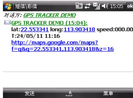
\*When lost fix to satellites, the message will include the last known GPS position and the LAC code of current position as well.
